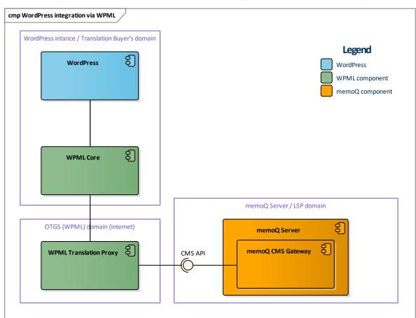
Figure 2. Architectural view of WordPress-memoQ integration via WPML Translation Proxy
