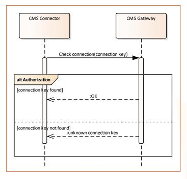
Figure 9. Collaboration protocol of performing connection health check
